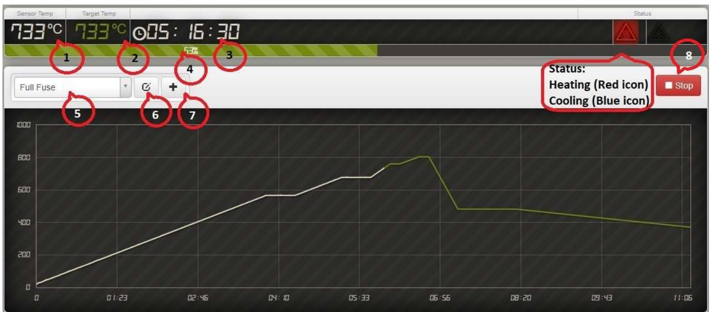
Figure 2. Thermocontroller WEB Interface. (1) Current temperature; (2) Currently programmed temperature; (3) Remaining time until the program run ends; (4) Completion progress; (5) Pre-set programs list; (6) Edit selected program; (7) Add/save new pre-set program; (8) Start/Stop button.
